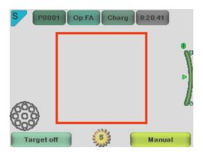
3. Default Display window when FA optics is attached using AF Assist mode. Diopter scale is automatically adjusted, Image can be captured when shutter button is pressed half a way.
