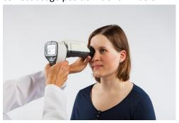
10. Still image is captured by pressing the shutter key all the way down. Video is captured by keeping shutter down. Taken image is displayed on screen until user clears the image by pressing shutter, left or right soft key. Image can be zoomed in instant preview by pressing middle key. There are four zoom levels. Pressing middle key activates the next level. Move around the image by using arrow keys.
