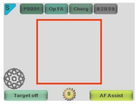
4. Default Display window when FA optics is attached using MF Assist mode. Diopter scale is manually adjusted, Image can be captured when shutter button is pressed half a way.
