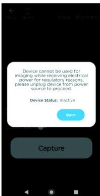
While the device is plugged in, imaging mode is not accessible. The user will see “Device cannot be used for imaging while receiving electrical power for regulatory reasons. Please unplug device from power source to proceed.” The user must unplug the device to image.
