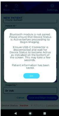
When the device is Inactive, imaging mode is not accessible. The user will see “Bluetooth module is not paired. Please ensure that Device Status is Active before proceeding to Begin Imaging. Ensure USB-C Connector is disconnected and wait for Device Status to become Active as indicated on the bottom of the screen. This may take a few seconds. Patient information has been saved.” Connect to Bluetooth or unplug the device to image.
